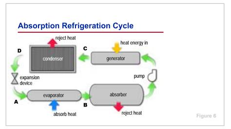
There are two fundamental differences between the absorption refrigeration cycle and the vapor-compression refrigeration cycle. The first is that the compressor is replaced by an absorber, pump, and generator. The second is that, in addition to the refrigerant, the absorption refrigeration cycle uses a secondary fluid, called the absorbent. The condenser, expansion device, and evaporator sections, however, are the same.
